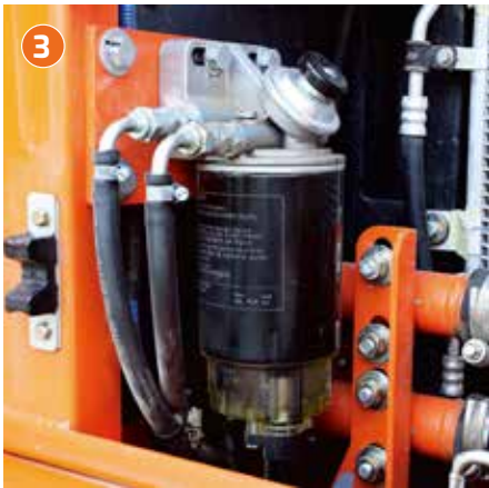
FUEL FILTER High efficiency fuel filtration is attained by the use of multiple filters, including a fuel pre-filter fitted with a water separator that removes most moisture from the fuel.
