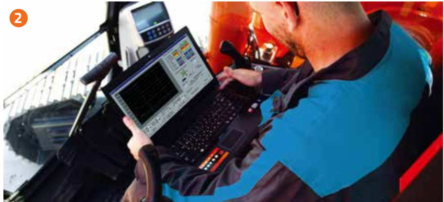
PC MONITORING A PC monitoring function enables connection to the EPOS™ system. Thus, various parameters can be checked during maintenance, including pump pressures, engine rotation and engine speed.
