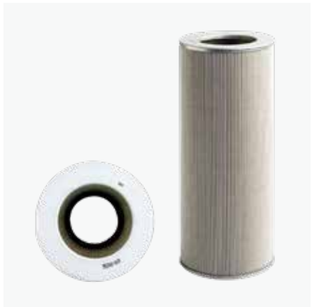
HYDRAULIC OIL RETURN FILTER The protection of the hydraulic system is more effective, using glass fiber filter technology in the main oil return filter. This means that with more than 99.5% of foreign particles filtered out, the oil change interval is increased.
