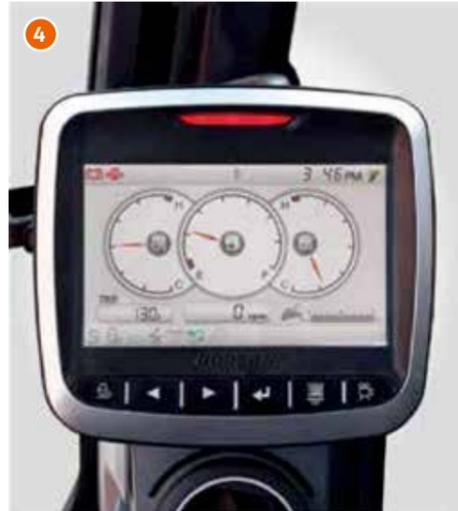
Another customer convenience feature is the **8 inch LCD monitor that provides operators with various kinds of information about the machine state.**
