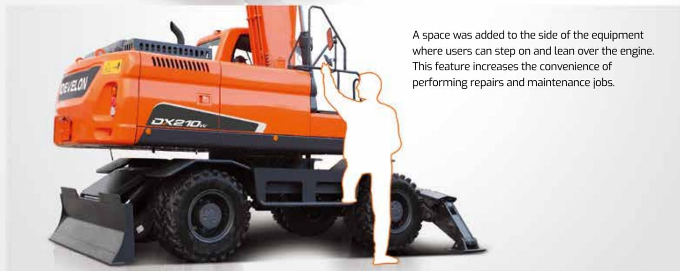
A space was added to the side of the equipment where users can step on and lean over the engine. This feature increases the convenience of performing repairs and maintenance jobs.
